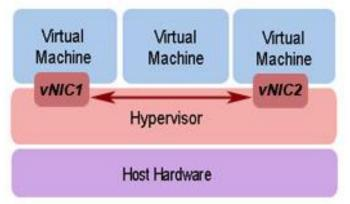
Figure 5: VMs communication on one a physical host.
