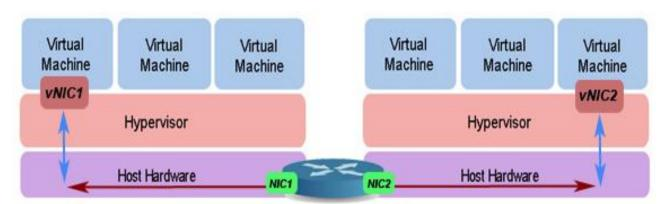
Figure 6: VMs communication on two physical hosts.
